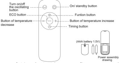
Control range of remote controller The remote controller control can be normally used within 5 meters in front of the product and in the left and right angles of 30 degrees. Please use a manganese or alkaline battery of type "AAA" and do not use a non-recycla ble battery.
